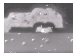
Fig. 1 – SEM cross-section of Integra's 0.5µm GaN HEMT chip with double field plate design.
