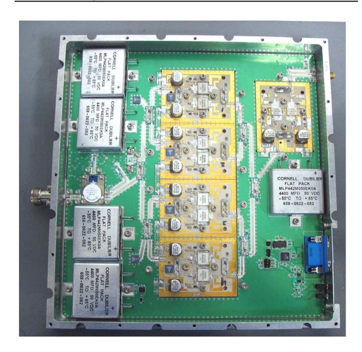
Figure 1. 3.1-3.5GHz, 2-stage, 650 Watt Pulsed Power Amplifier
