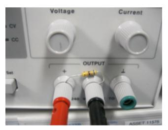
FIGURE 2: Configuring the gate power supply to both sink and source gate current.
