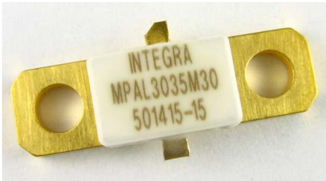
Fig. 7. Example of a miniaturized power amplifier using LDMOS technology. The MPAL3035M30 produces more than 30W of output power from 3.0 – 3.5 GHz. The package flange is 230 mils x 800 mils.
