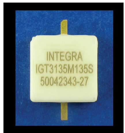
▲ Fig. 2 S-Band (3.1 to 3.5 GHz) 135 W GaN transistor internally matched to 50 \Omega . Package size is 0.4" \times 0.4".
