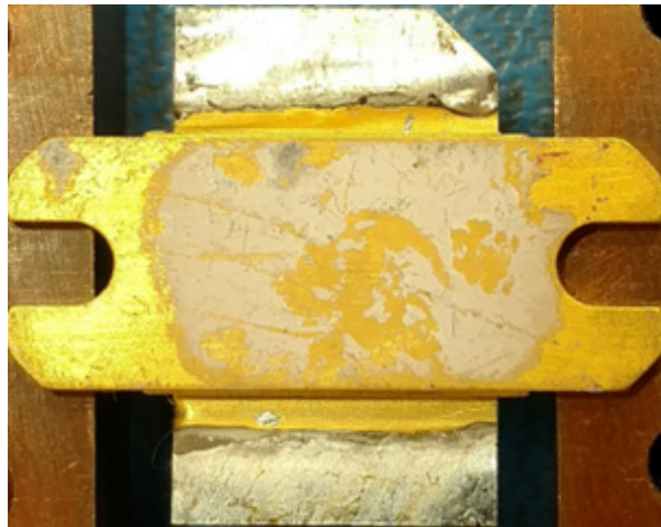
FIGURE 2: Example of a transistor that failed due to incorrect application of silicone grease.
