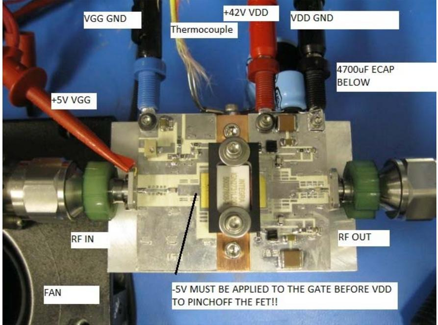
Figure 3- Test Fixture on RF Test Bench (typical)
