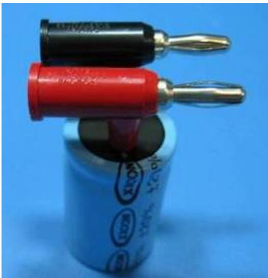
Figure 2- Drain Supply Filter Cap Provided 4700uF (typical)
